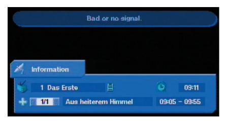
"Weak or no signal" indicates that an error has occurred in the receiving system or in the receiver settings, or that the transponder is not sending. The channel message then shows a satellite antenna instead
